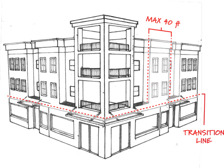
FIGURE 9.1 BUILDING ORIENTATION & MASSING
